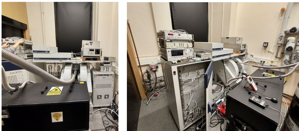
Figure 2. Example of an arrangement of a mobile laser table in front of the E580 spectrometer in F11.
